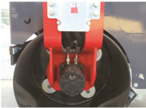
Hydraulic vibration is driven by imported motor
