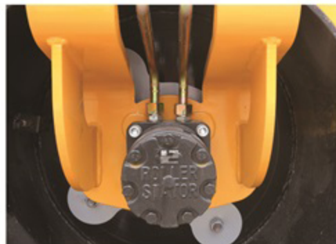
Hydraulic motor, double drum driving
