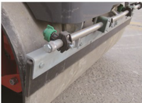
Double drum water spraying, scraper cleaning
