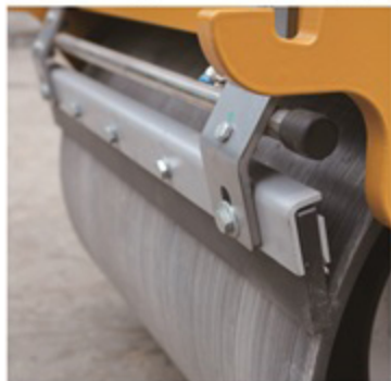
Double drum water spraying scraper cleaning
