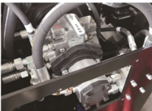
Imported hydraulic variable plunger pump
