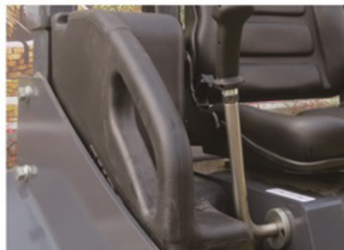
Large plastic water tank free from corrosion and convenient for water spraying
