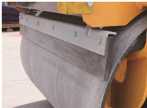
Double drum water spraying scraper cleaning
