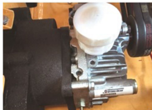
Original imported hydraulic pump variable speed
