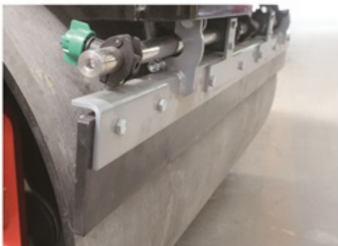
Double drum water spraying, scraper cleaning
