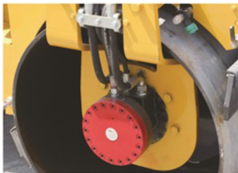
Imported plunger motors, double drums hydraulic driving
