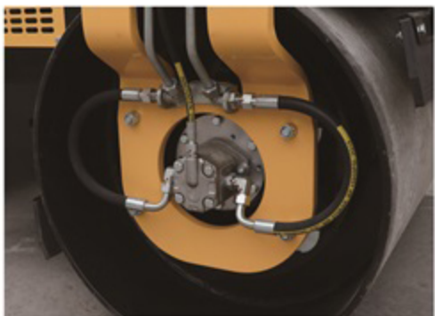
Hydraulic vibration is driven by impored motor
