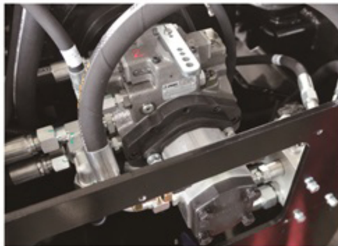
Imported hydraulic variable plunger pump
